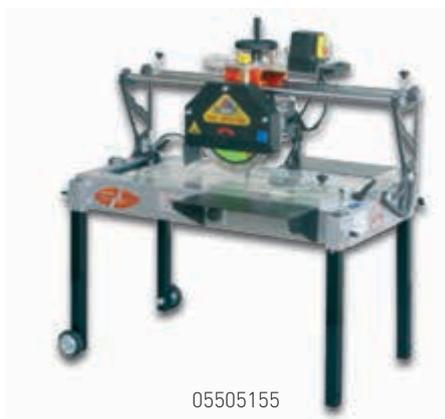
Aluminium base workbench; cutting head sliding on chrome and adjusted bars, manual feed by using appropriate handle, vertical movement via handwheel; head tilt to 45°; removable legs; stabilising bars.
