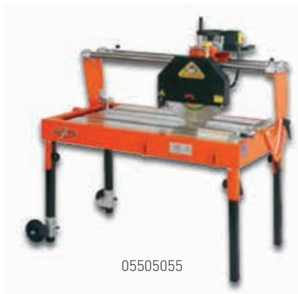
Iron base workbench; cutting head sliding on chrome and adjusted bars, manual feed by using the appropriate handle, vertical movement via the handwheel; head tilt to 45°; removable legs.
