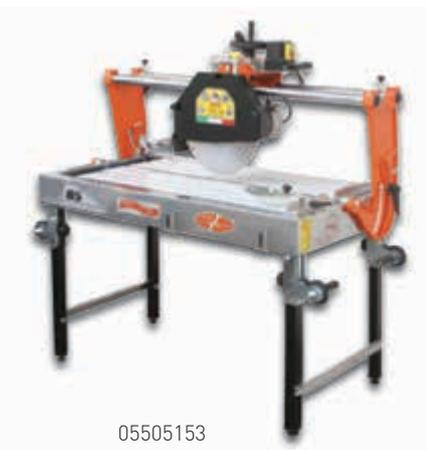
Aluminium base workbench; cutting head sliding on chrome and adjusted bars, manual feed by using appropriate handle, vertical movement via handwheel; head tilt to 45°; removable legs.
